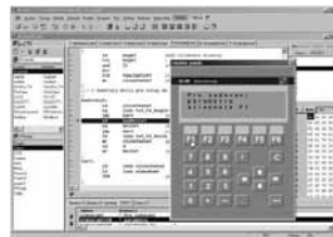
MOSAIC – the programming package based on the IEC 61131-3 standard enables to create application program in ST, IL, LD and FBD language as one project or group of projects.
