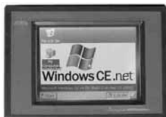
HMI products are represented by TEMPO – panel computer powered by Windows CE.net and Linux
